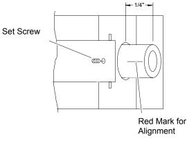
Figure 6-5. Lamp Alignment
